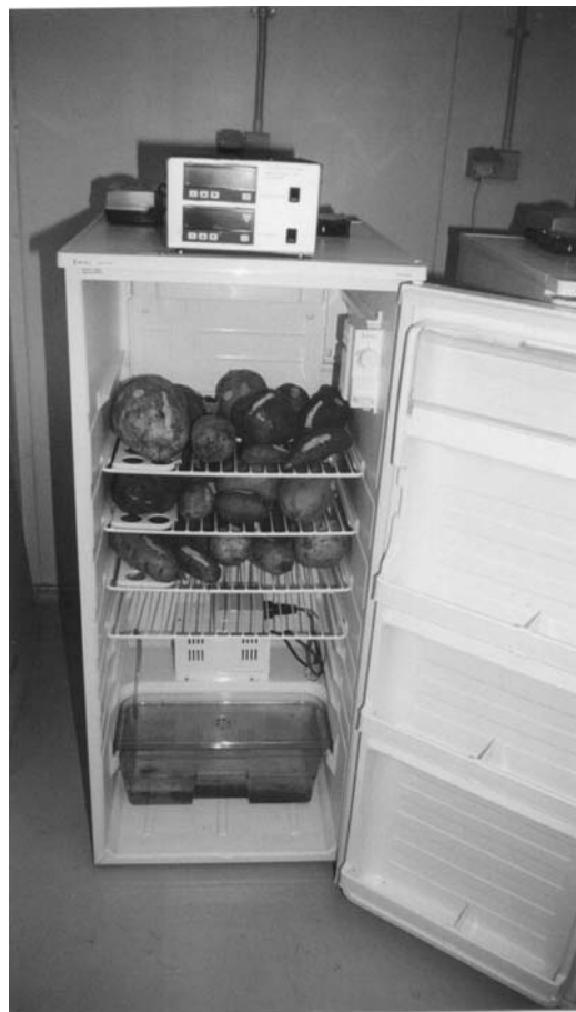
Figure 2.2 A humidity control chamber containing sweetpotatoes for screening.
