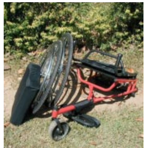
The low-tech WorldMade wheelchair design with folding backrest and removable wheels.
